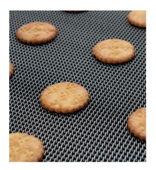
This belt is recommended for large, high-performance equipment (speeds of up to 30 m/min). The spaces between the mesh allow excellent air circulation during cooking.
